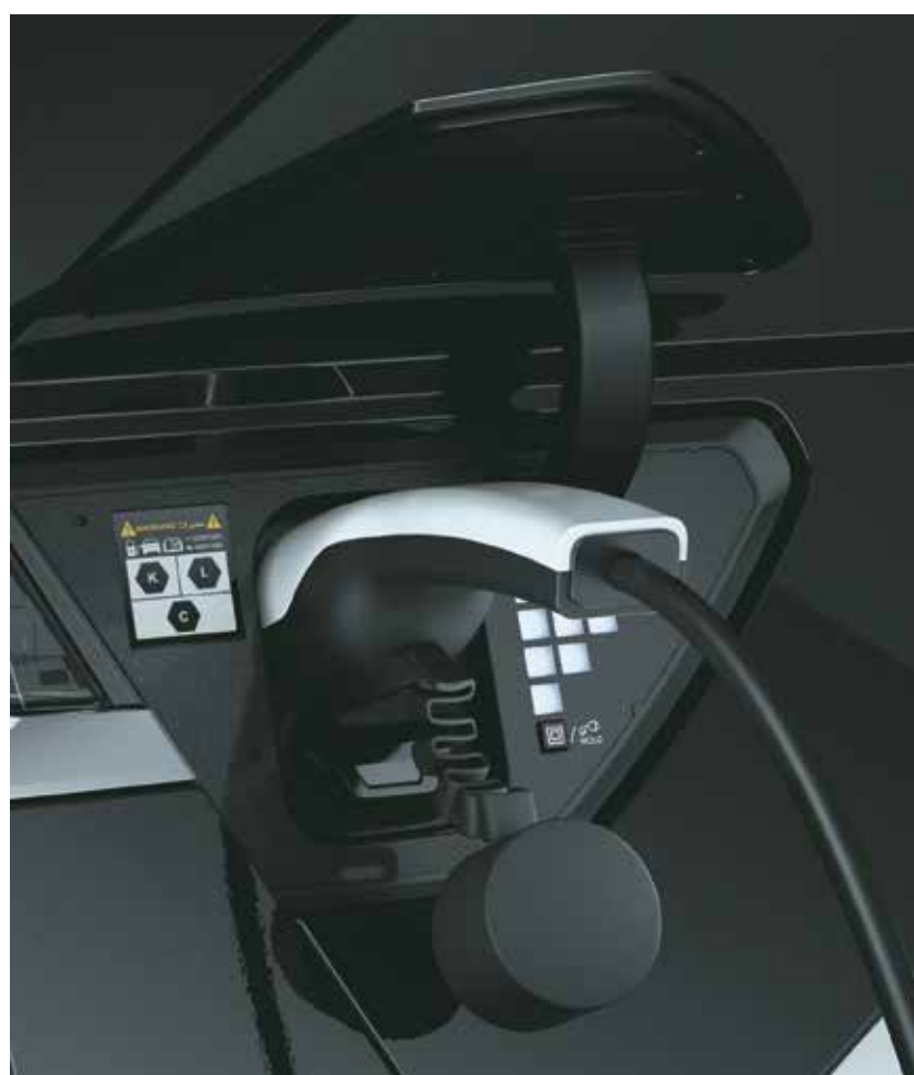
Home charging (11 kW AC wallbox charger)
