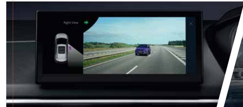
BLIND VIEW MONITOR Watchful eye for hidden views. Ensure a safe drive with a clear side view on the screen during turns
